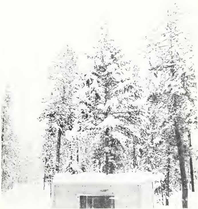
Figure W-6. -- Mounted on scales, this 15-foot Engelmann spruce intercepted 36 pounds of snow during one snowstorm -- 7-1/2 inches of snow, with a water equivalent of 0.41 inch, fell in the storm.
